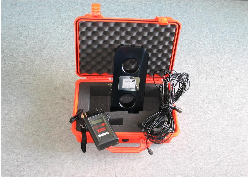
The Digilink is a portable load cell package combining high quality, accuracy and reliability in a compact low weight unit; the Digilink is supplied complete with a remote hand held display/control module, 10metres lead, leather carry case, battery charger and test certificate all housed in a rugged waterproof case.
