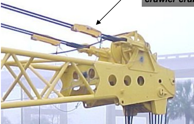
LOADWISE Clamp-On Dynamometers fitted to the pendant ropes on a crawler crane
